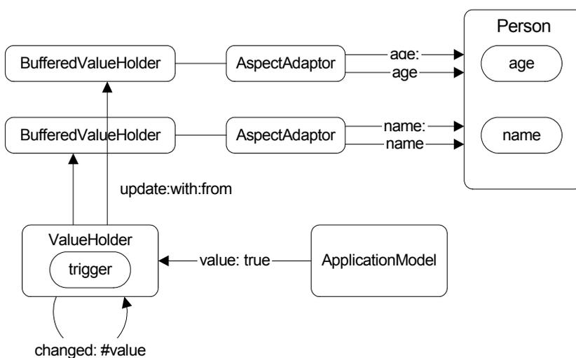
**Figure 24-6.** The BufferedValueHolder mechanism.
