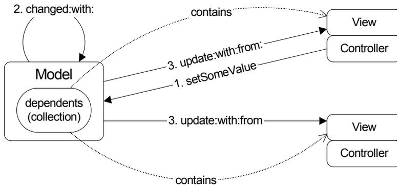
Figure 23-2. Model-View-Controller interactions.
